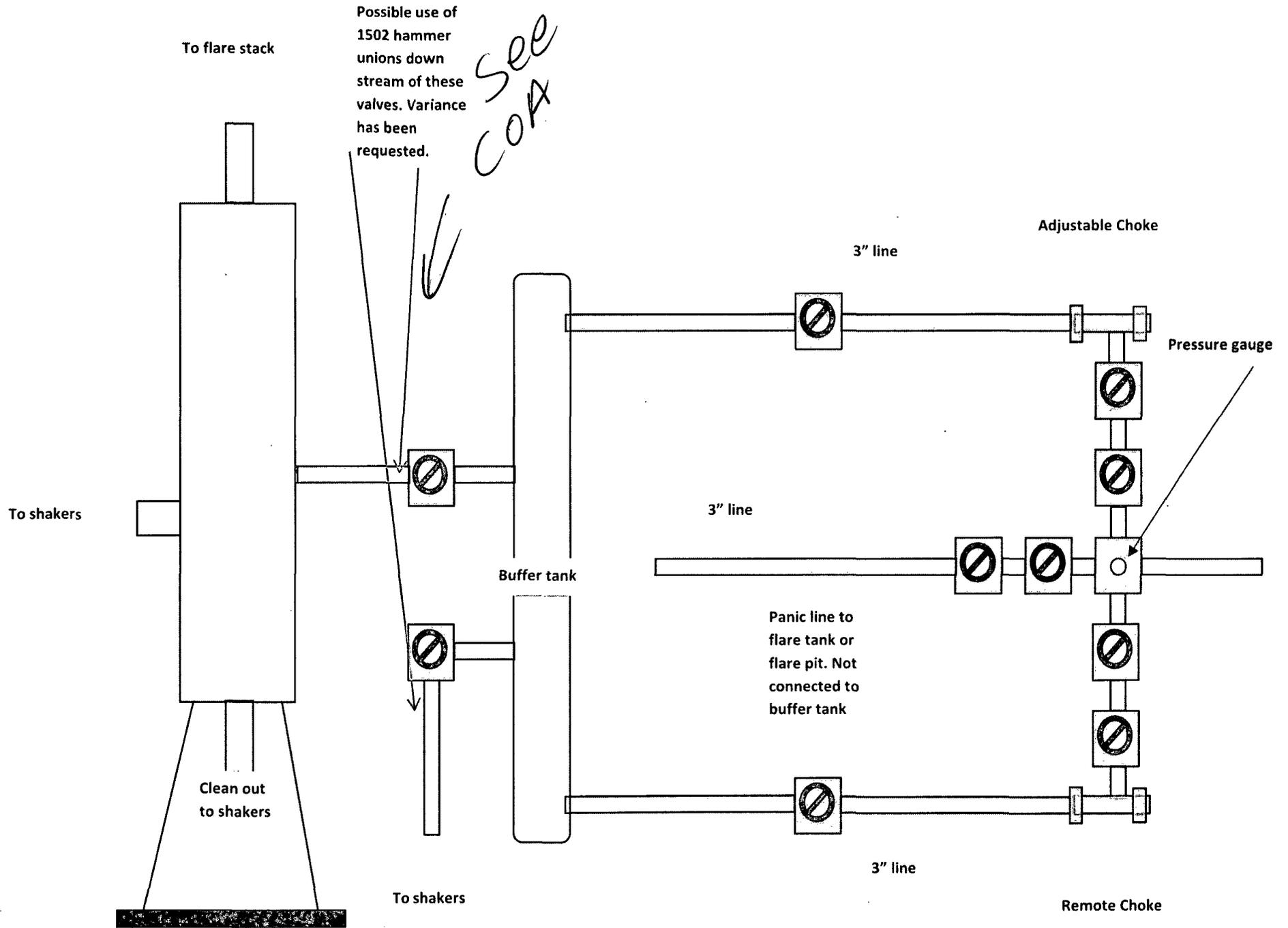
**BOP, Choke Manifold and Process Flow Diagrams - Hamon Fed Com A #1H (See Patriot Rig 5 Choke Manifold Equipment Diagram for greater detail)**
