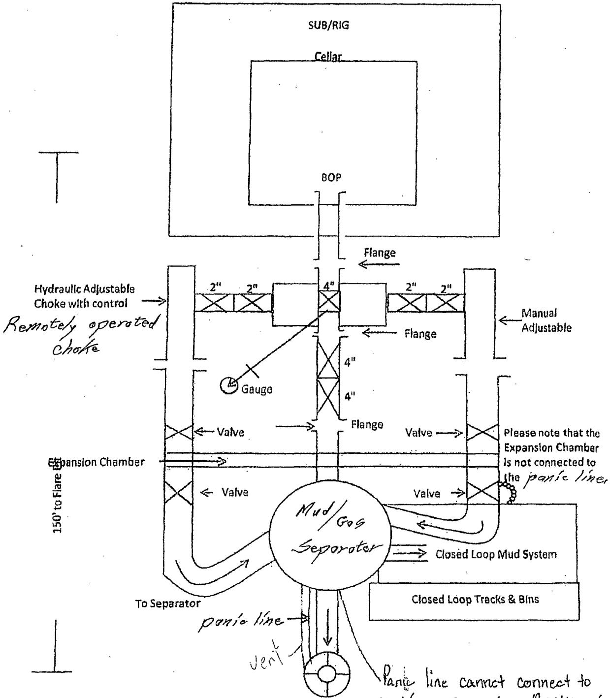
*Panic line cannot connect to mud/gas separator. Additional vent line is needed for mud/gas separator.*
