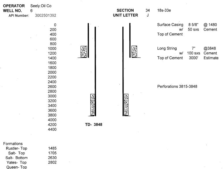
Operator Seely D. / Company Surt, Sqz cnt Well Name No. Carkburn Fed 6 API 300250/392 Hole Size per FCP 350 2310 N(S) 2319 E/W Sec. 34 Cnt, sxs 50 Toc ? TWN 175 RNG 33 E Rustler 1485 (sg.sz <u>85/8</u> TD 1398 War Eag 1348 T/SALT 1705 B/SALT 2630 SQZ cm. f T/Salt shoe Hole Size\_\_\_\_ R-111-P A.+@1755 CAVE/KARST Cond. SXS 100 TOC ? FORMATION TOPS: Yates 2802 Queen 3800 LOOC Tay 2570 SOZ cmt T/yt B/self Perf 2852 DVT: PERFORATIONS: WAL To-9 3700 3848 3795 Cg Sz 7" TD <u>3848</u> PBTD . 3848
