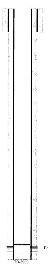
11" hole @ 369' 7-5/8" csg @ 369' w/ 200sx-TOC-Surf-Circ
