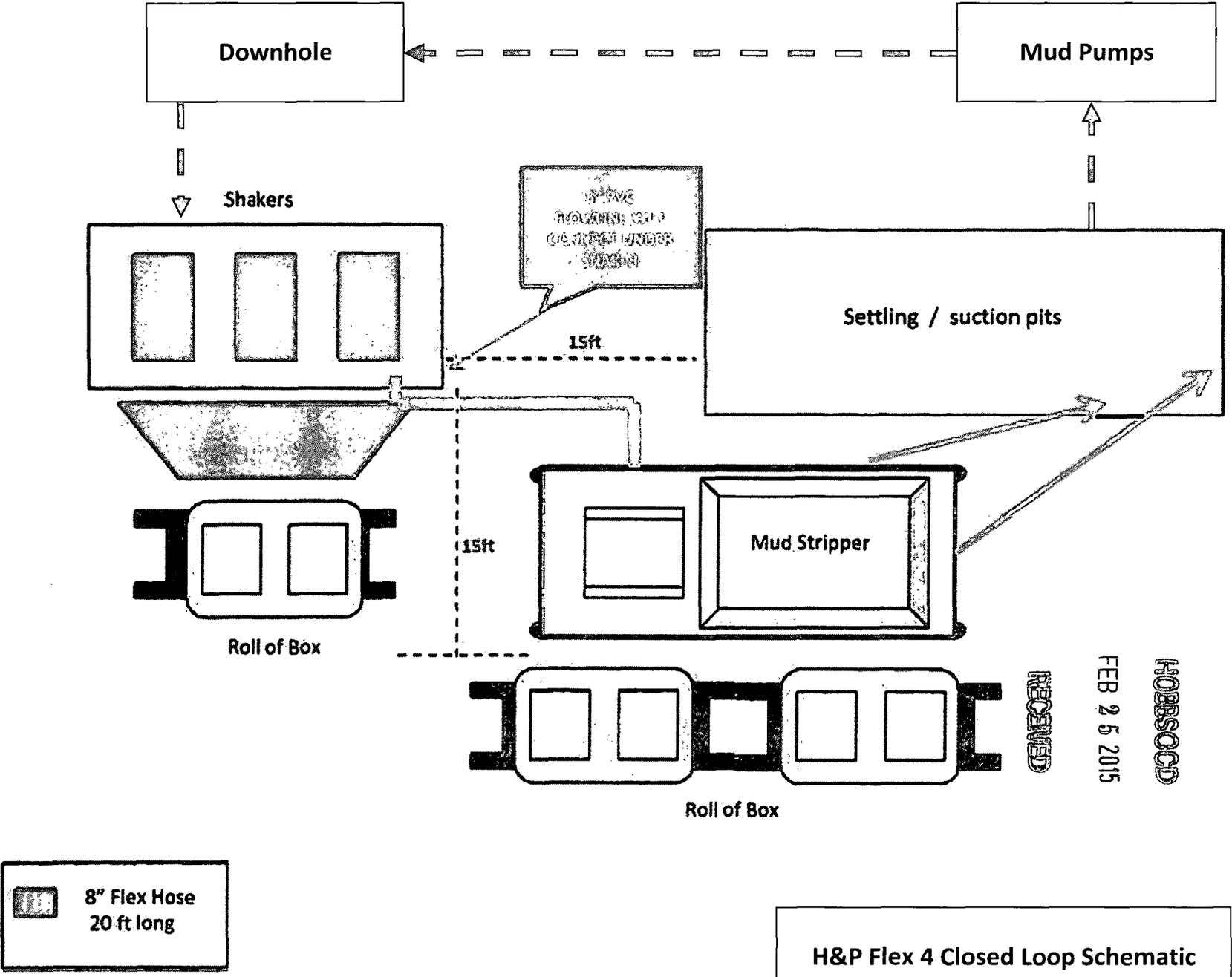
H&P Flex 4 Closed Loop Schematic
