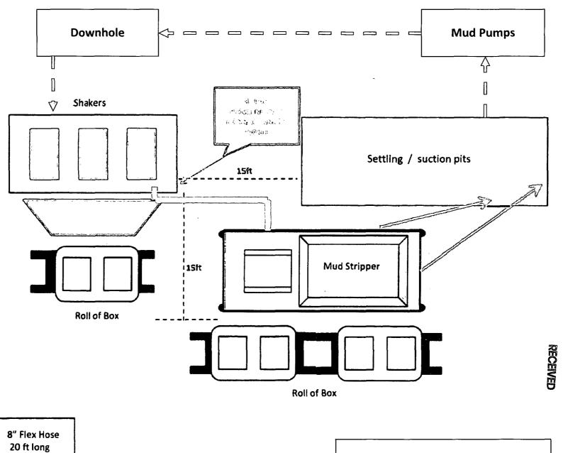
**H&P Flex 4 Closed Loop Schematic**
