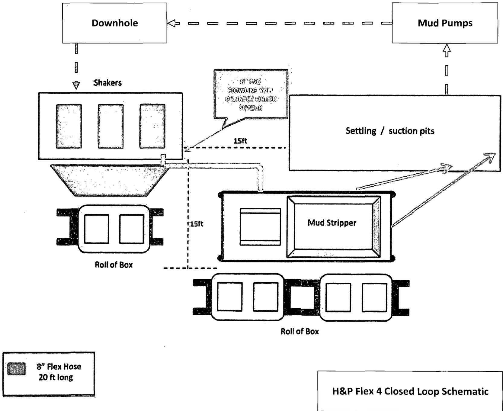
H&P Flex 4 Closed Loop Schematic
