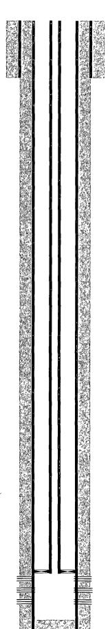
12-1/4" hole @ 362' 8-5/8" csg @ 362' w/ 300sx-TOC-Surf-Circ
