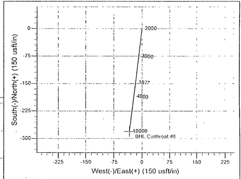
1650 FNL and 1650 FEL are Hard Lines. The well can be south, west, or southwest of these hard lines but not north, east, or northeast. From the BHL the well is 25' south of the north hard line and 25' west of the east hard line
