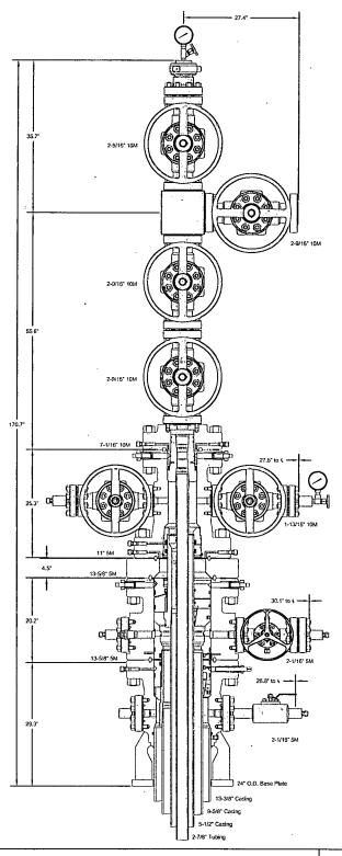
CHEVRON USA, INC. **DELAWARE BASIN** 19MAR13 VJK DRAWN 13-3/8" x 9-5/8" x 5-1/2" x 2-7/8" 10M SH2/Conventional APPRV KN 19MAR13 Wellhead Assembly, With DSA, T-EBS-F Tubing Head, FOR REFERENCE ONLY AE23705 T-EN Tubing Hanger and A5PEN Adapter Flange
