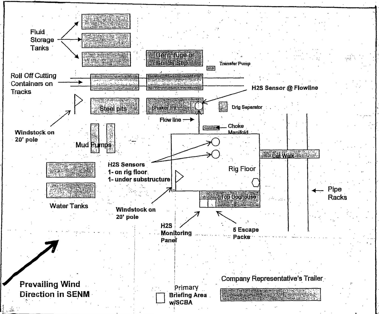
H<sub>2</sub>S EQUIPMENT SCHEMATIC
