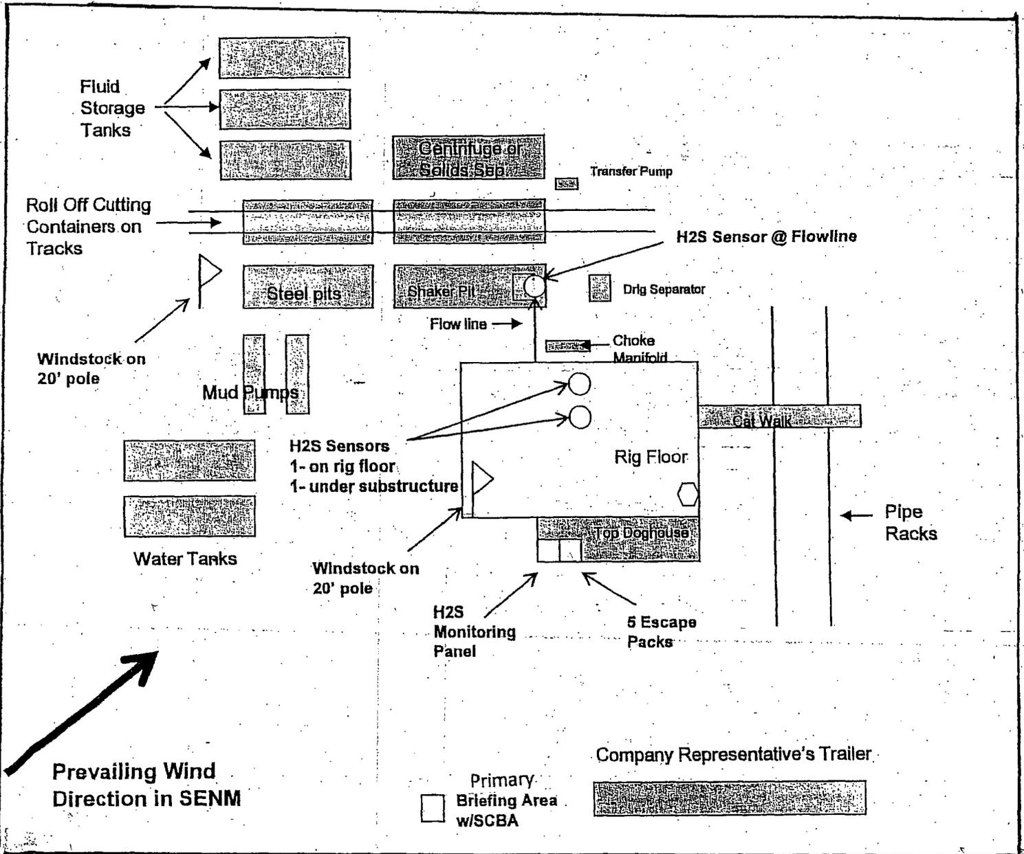
H<sub>2</sub>S EQUIPMENT SCHEMATIC
