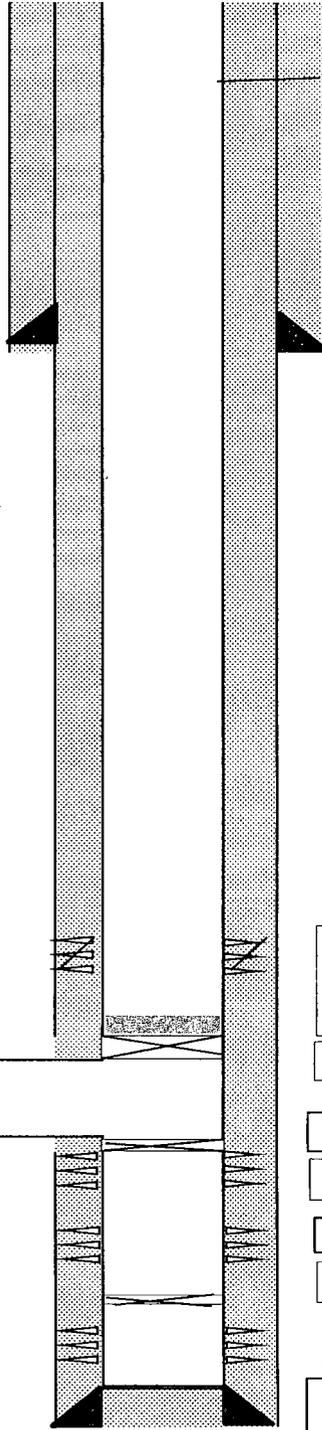
0-647' gross interval. Casing leak identified during TA attempt. Exact location not pinpointed.
