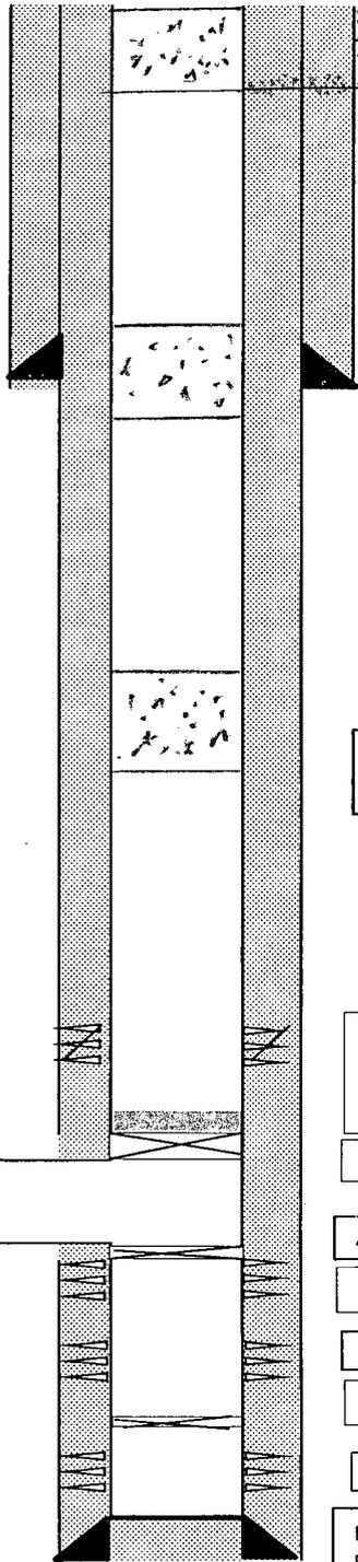
0-647' gross interval. Casing leak identified during TA attempt. Exact location not pinpointed.
