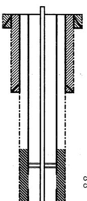
Casing swaged and milled out to 4-5/8", 7007' - 7325' (9/92) Casing swaged out to 4-5/8", 7339' - 7648' (08/05)
