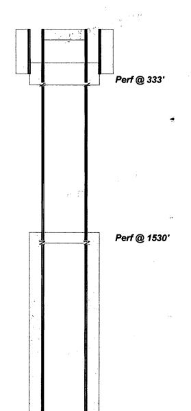
11" hole @ 283' 8-5/8" csg @ 283' w/225sx-TOC-Surf-Circ
