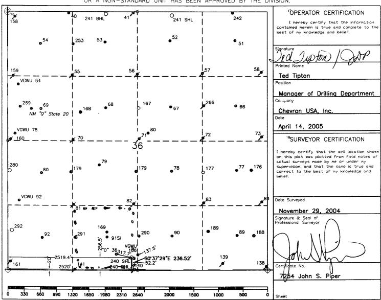
○ = Staked Location • = Producing Well 💉 = Injection Well 💠 = Water Supply Well 💠 = Plugged & Abandon Well
