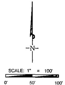
ALL BEARINGS, DISTANCES, AND COORDINATE VALUES CONTAINED HEREON ARE GRID BASED UPON THE NEW MEXICO STATE PLANE COORDINATE SYSTEM, EAST ZONE OF THE NORTH AMERICAN DATUM 1927, U.S. SURVEY FEET
