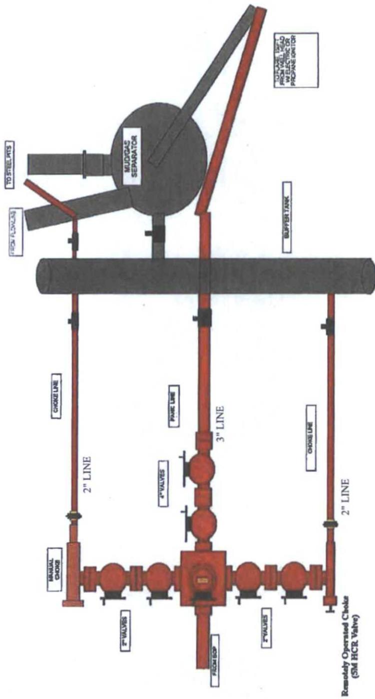
Figure 12 (Revised): BOP Manifold Schematic
