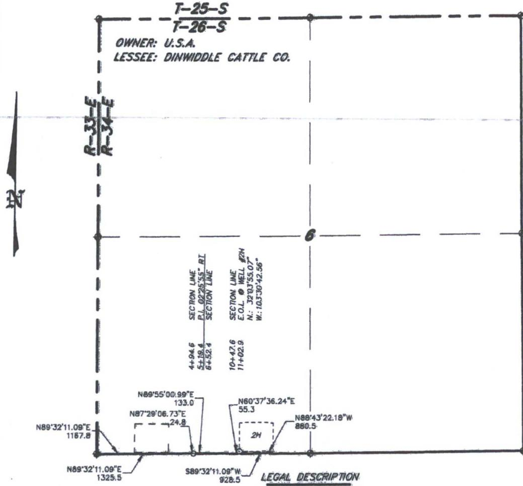
A STRIP OF LAND 30.0 FEET WIDE, LOCATED IN SECTION 6, TOWNSHIP 26 SOUTH, RANGE 34 EAST, N.M.P.M., LEA COUNTY, NEW MEXICO AND BEING 15.0 FEET LEFT AND RIGHT OF THE ABOVE PLATTED CENTERLINE SURVEY.
