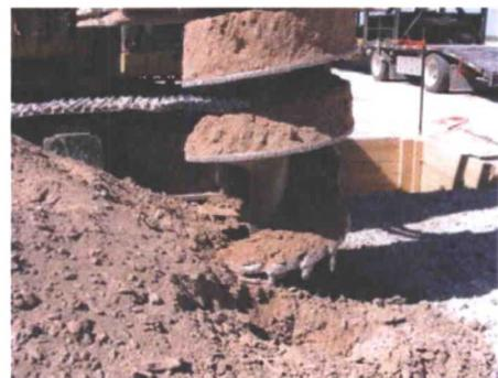
Over the next 2.5 hours the boring was advanced to a total depth of 120 feet by removing approximately 1 to 1.5 feet of material per trip into the hole. Mr. Littlejohn carefully inspected each auger for the appearance of moisture in the soil prior to it being spun off
