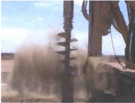
The photograph to the left was taken from the soil recovered at a depth of 98 feet as it is being spun from the auger. This photograph demonstrates the lack of moisture in the cuttings. It is believed that any potential moisture from the bottom or walls of the boring would have been easily identified during the drilling process as each trip into the hole should contact wet soil if it is present at any depth.
