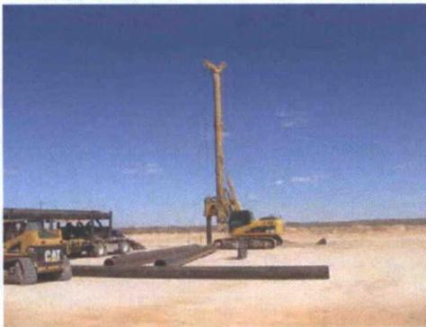
On February 27, 2013 I witnessed the drilling of the rat hole at the Mogi 9 #1H site. Ready Drill LLC of Monahans, Texas performed the work using a track-mounted 30-inch auger drilling rig as shown in the adjacent photograph.
