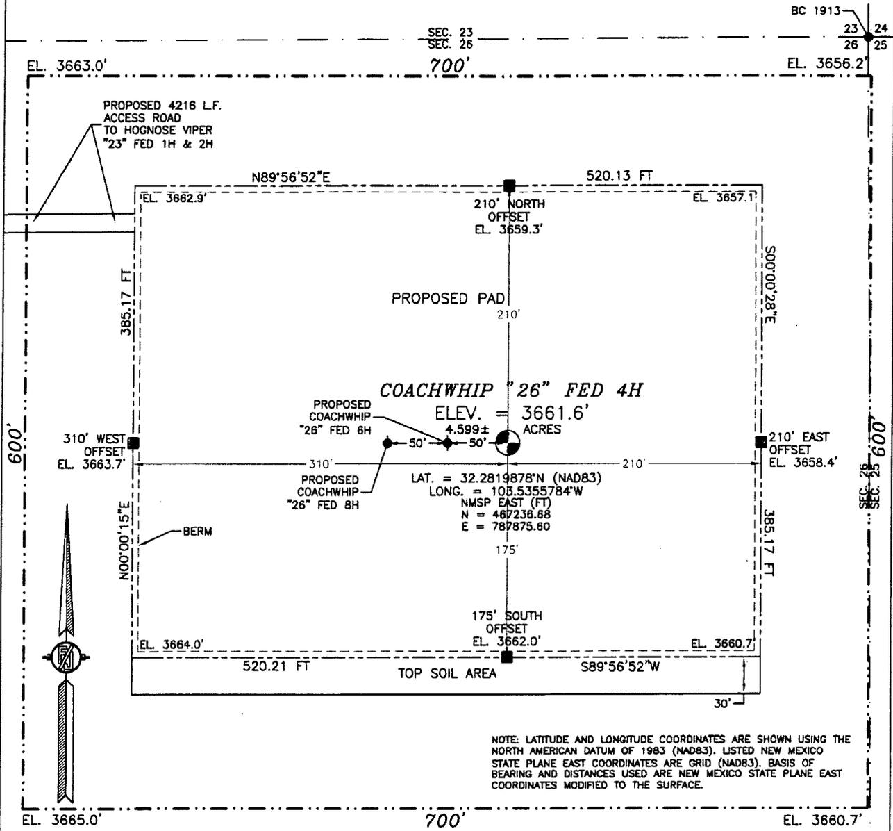
NOTE: LATITUDE AND LONGITUDE COORDINATES ARE SHOWN USING THE NORTH AMERICAN DATUM OF 1983 (NAD83). LISTED NEW MEXICO STATE PLANE EAST COORDINATES ARE GRID (NAD83). BASIS OF BEARING AND DISTANCES USED ARE NEW MEXICO STATE PLANE EAST COORDINATES MODIFIED TO THE SURFACE.
