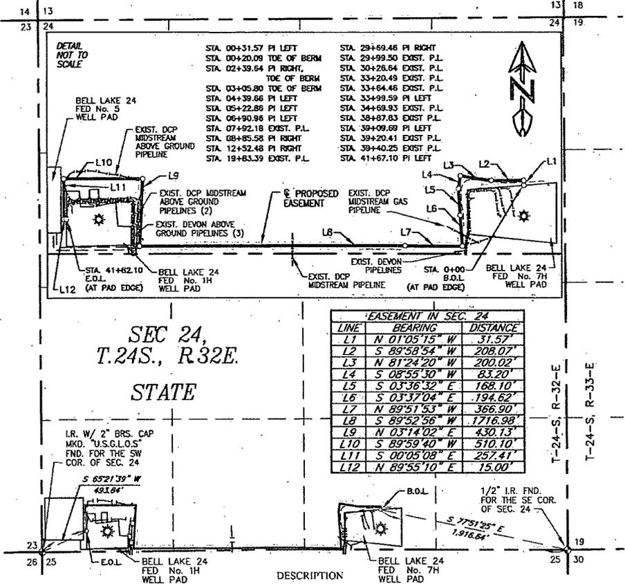
A 30' wide pipeline easement for a 6 inch Poly pipe production flowline to carry oil, gas and water crossing state land in Section 24, Township 24 South, Range 32 East, N.M.P.M., Lea County, State of New Mexico and being 15' on each side of the following described centerline.
