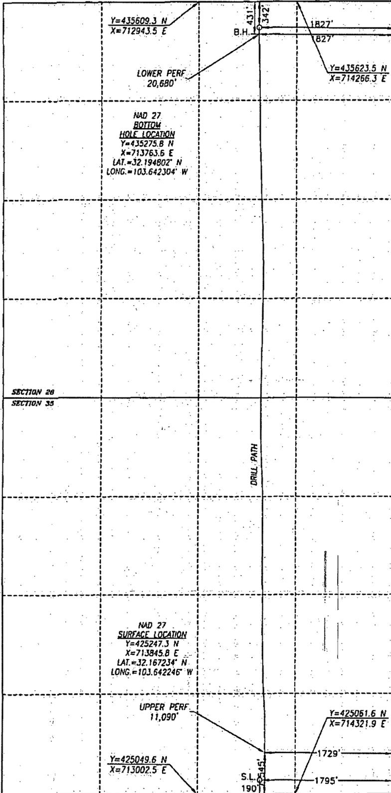
BOREPATH SHOWN HEREON IS BASED ON A DIRECTIONAL SURVEY REPORT PROVIDED BY COG OPERATING, LLC FOR THE EIDER FEDERAL #2H SUPPLIED TO HARCROW SURVEYING, LLC ON MARCH 31, 2016.
