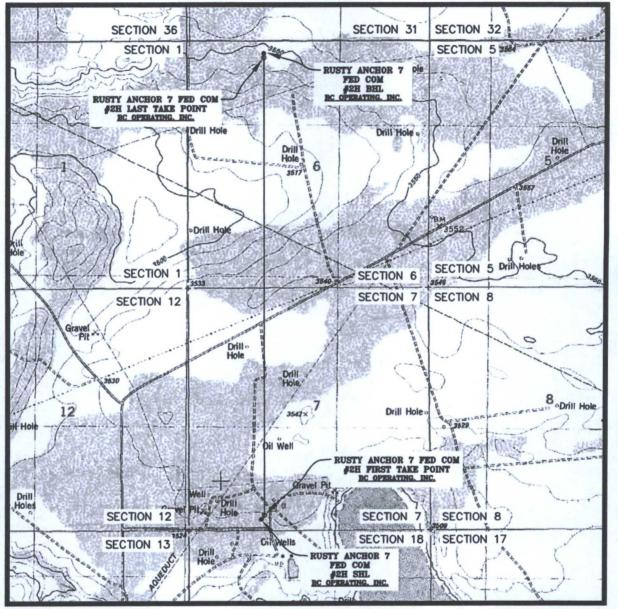
SEC. 7 TWP. 20-S RGE. 33-E SURVEY: N.M.P.M. COUNTY: LEA DESCRIPTION: 236' FSL & 1613' FWL ELEVATION: 3532' OPERATOR: B.C. OPERATING, INC. LEASE: RUSTY ANCHOR 7 FED COM U.S.G.S. TOPOGRAPHIC MAP: LAGUNA GATUNA, N.M. SCALE: 1" = 2000' CONTOUR INTERVAL = 5'
