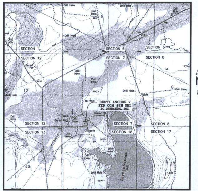
SEC. 7 TWP. 20-S RGE. 33-E SURVEY: N.M.P.M. COUNTY: LEA DESCRIPTION: 236' FSL & 1613' FWL ELEVATION: 3532' OPERATOR: B.C. OPERATING, INC. LEASE: RUSTY ANCHOR 7 FED COM U.S.G.S. TOPOGRAPHIC MAP: LAGUNA GATUNA, N.M. SCALE: 1" = 2000' CONTOUR INTERVAL = 5'
