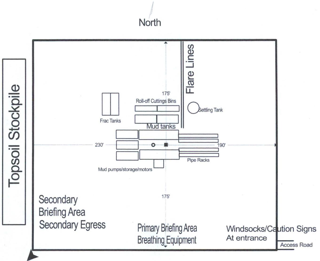
Alarms will be placed on the mud tanks, at the shale shaker, and on the rig floor. Windssocks will also be present on the top of the substructure and near the mud tanks.
