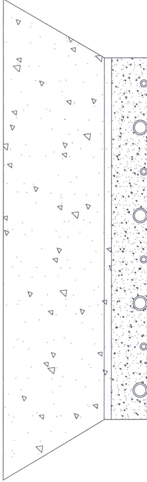
BACKFILL DIRT TO BE AS FREE OF ROCKS AND LARGE PARTICLES AS POSSIBLE
