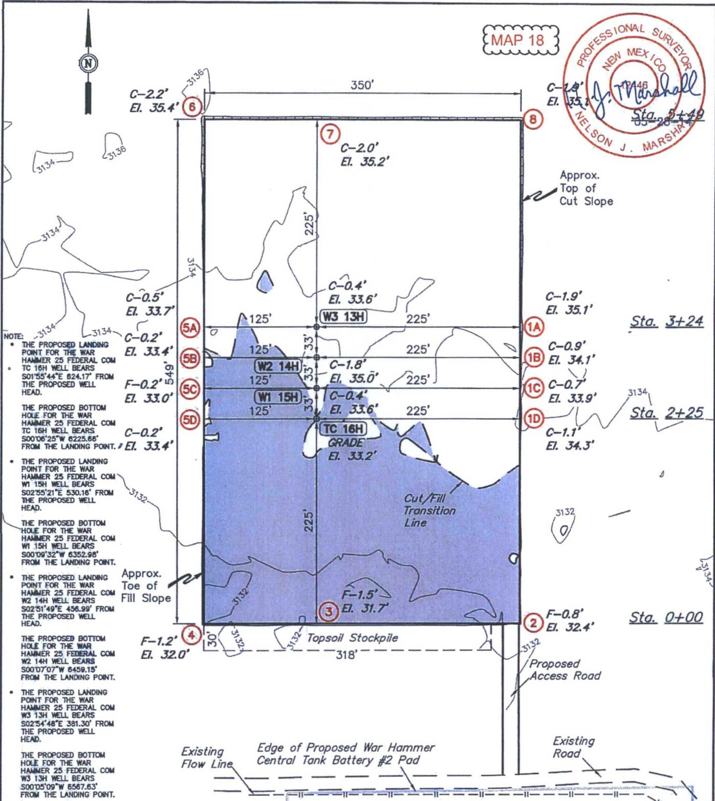
ELEV. UNGRADED GROUND AT TC 16H LOC. STAKE = 3133.2' FINISHED GRADE ELEV. AT TC 16H LOC. STAKE = 3133.2'
