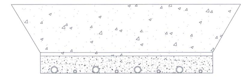
BACKFILL DIRT TO BE AS FREE OF ROCKS AND LARGE PARTICLES AS POSSIBLE FLOW LINE WILL BE 4" COATED STEEL PIPE w/ AN OPERATING PRESSURE UP TO 1480# PSI. GAS SUPPLY LINE WILL BE 2" STEEL PIPE w/ AN OPERATING PRESSURE UP TO 1100# PSI. SOFT FILL DIRT OR SAND WITH NO ROCKS OR SOLID PARTICLES GREATER THAN 1" IN CIRCUMFERENCE
