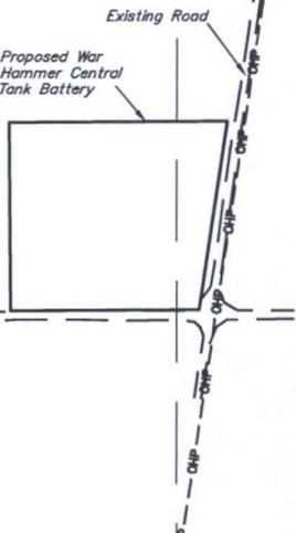
BEGINNING OF POWER LINE STA. 0+00 BEARS S53°29'19\"W 1321.70' FROM THE NORTHEAST CORNER OF SECTION 25, T26S, R32E, N.M.P.M.
