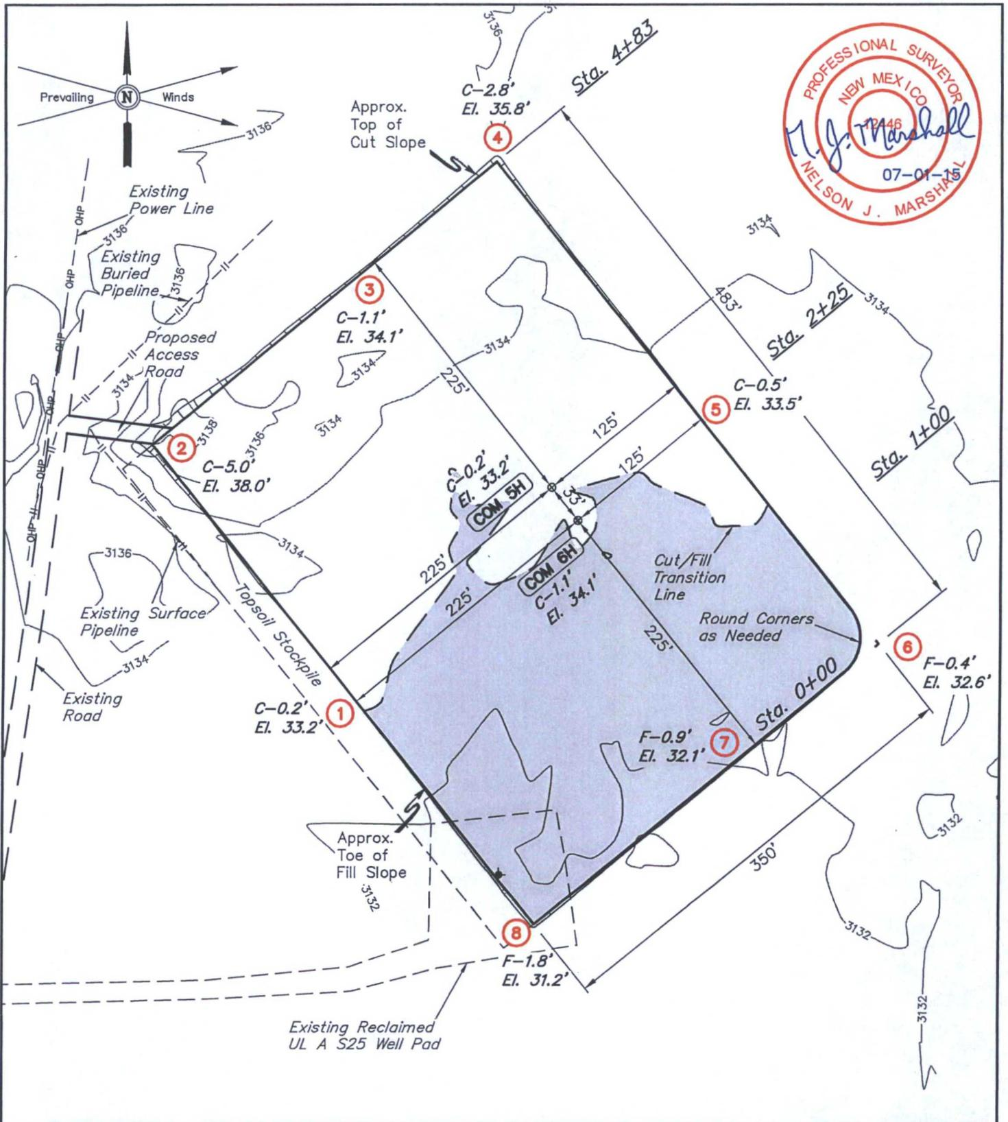
ELEV. UNGRADED GROUND AT W2 6H LOC. STAKE = 3134.1' FINISHED GRADE ELEV. AT W2 6H LOC. STAKE = 3133.0'
