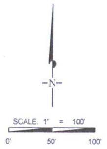
ALL BEARINGS, DISTANCES, AND COORDINATE VALUES CONTAINED HEREON ARE GRID BASED UPON THE NEW MEXICO STATE PLANE COORDINATE SYSTEM, EAST ZONE OF THE NORTH AMERICAN DATUM 1927, U.S. SURVEY FEET.
