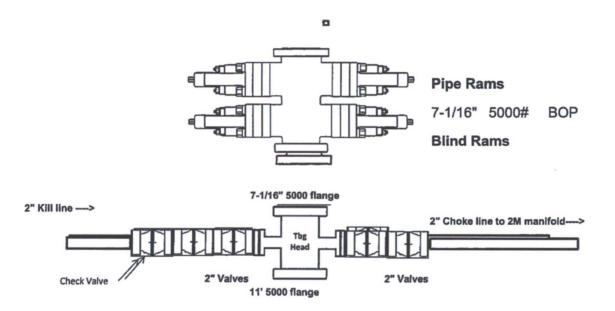
Note: Kill line and choke manifold will use BLM 2M configuration with 5000 psi WP components
