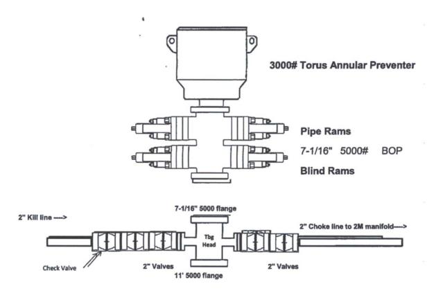
Note: Kill line and choke manifold will use BLM 2M configuration with 5000 psi WP components
