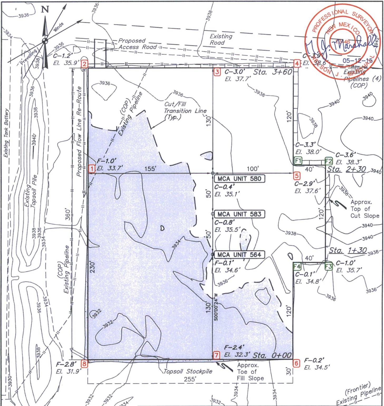
NOTE: Earthwork Calculations Require a Fill of 0.1' @ the MCA UNIT 564 Location Stake For Balance. All Fill is to be Compacted to a Minimum of 95% of the Maximum Dry Density Obtained by AASHTO Method t-99.
