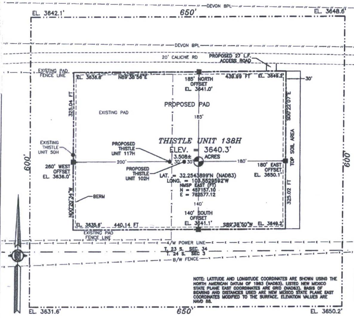
NOTE: LATITUDE AND LONGITUDE COORDINATES ARE SHOWN USING THE NORTH AMERICAN DATUM OF 1983 (NAD83). LISTED NEW MEXICO STATE PLANE EAST COORDINATES ARE GRID (NAD83). BASIS OF BEARING AND DISTANCES USED ARE NEW MEXICO STATE PLANE EAST COORDINATES MODIFIED TO THE SURFACE. ELEVATION VALUES ARE NAVD 88.
