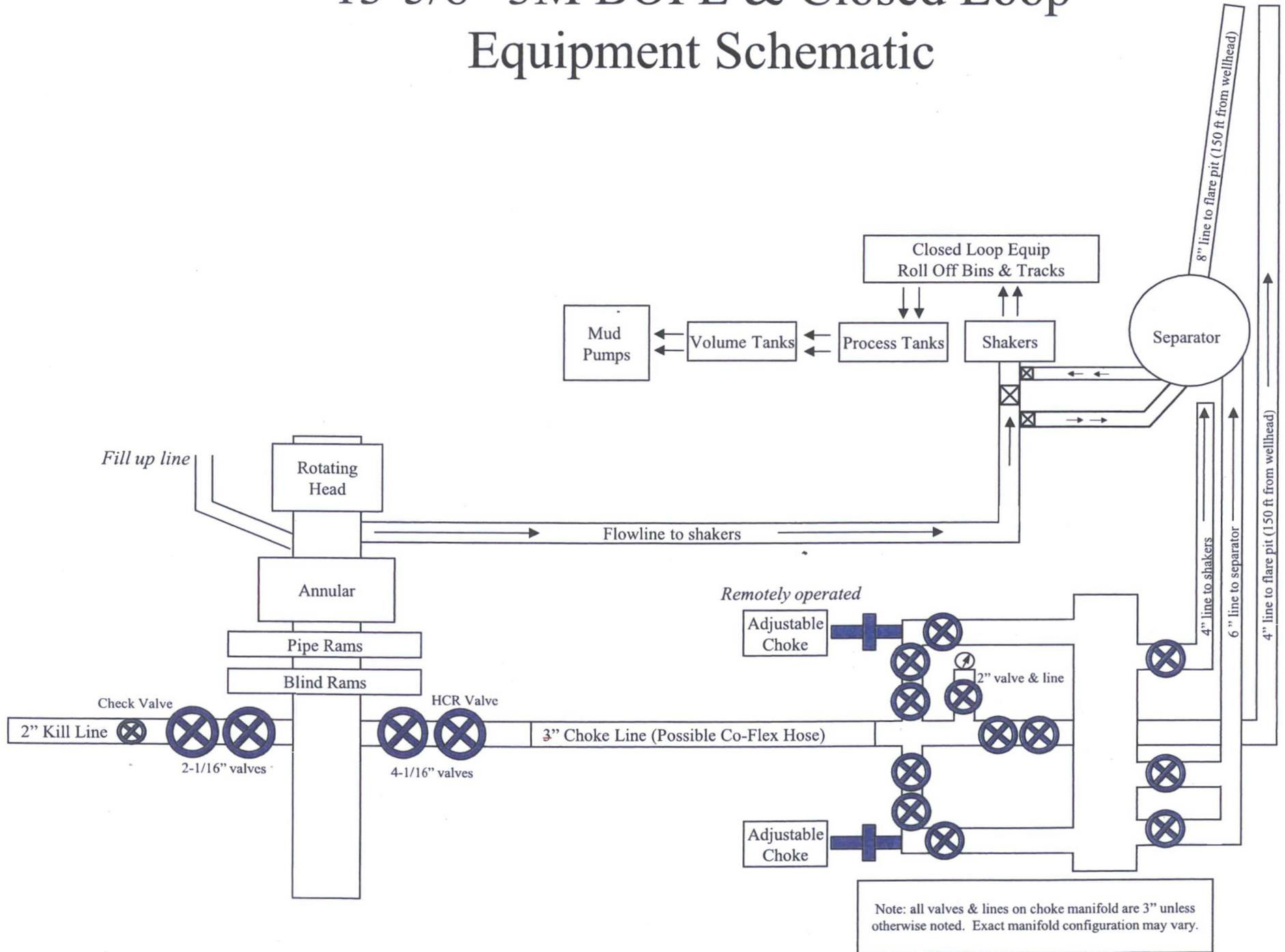
A multibowl wellhead may be used. The BOP will be tested per Onshore Order #2 after installation on the surface casing which will cover testing requirements for a maximum of 30 days. If any seal subject to test pressure is broken the system must be tested.
