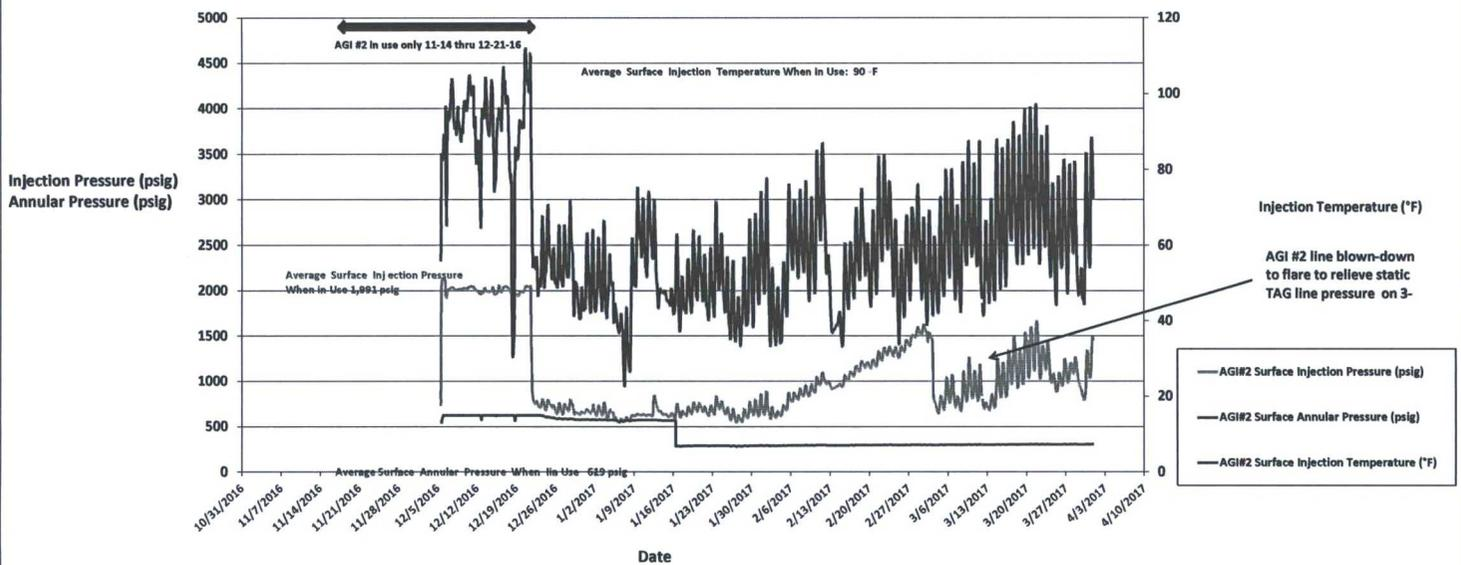
**Figure 4: Maljamar AGI #2 BH Injection Pressure & Temperature, Surface Annular Pressure**
