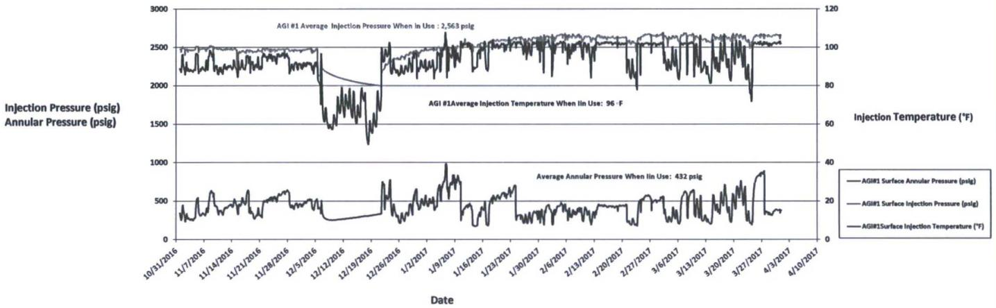
**Figure 3: Maljamar AGI #2 Surface Injection Parameters**
