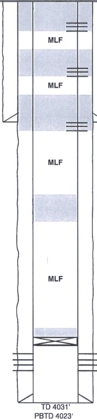
**Perf and Sqz. 150sx of Class "C" Cement from 400'-surface, Verify cement at surface. (FW/Surface.)**
