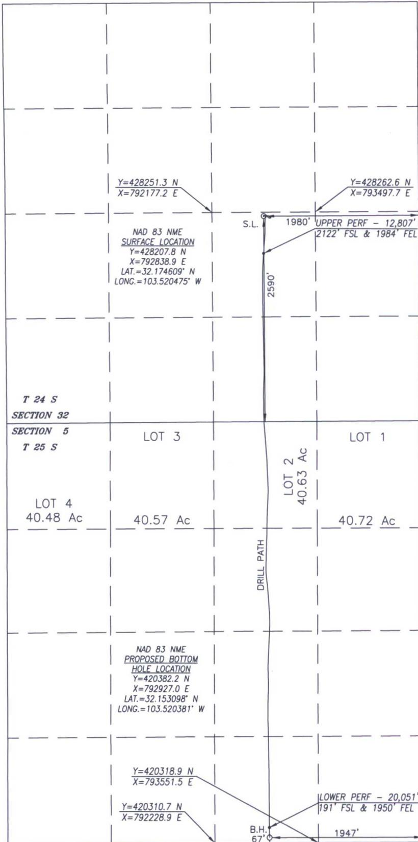
BOREPATH SHOWN HEREON IS BASED ON DIRECTIONAL SURVEY REPORT PROVIDED BY COG OPERATING, LLC FOR THE SKULL CAP FEDERAL COM #22H SUPPLIED TO HARCROW SURVEYING, LLC ON MARCH 2, 2017
