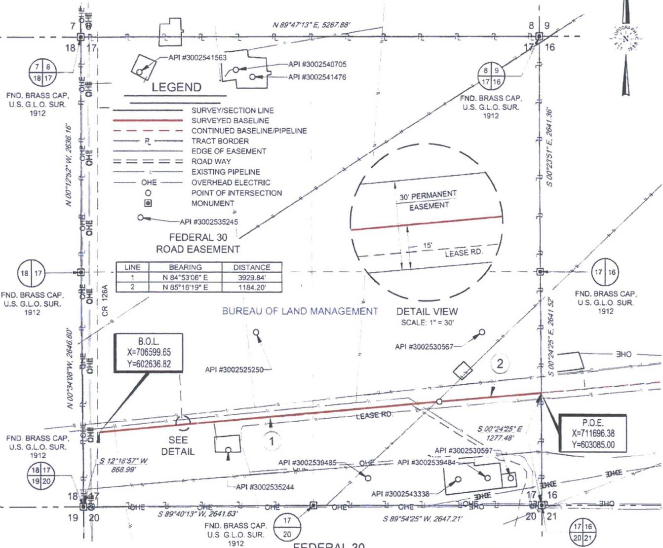
Being a proposed road easement being 30 feet in width, 15 feet left, and 15 feet right of the above platted centerline total line footage containing 5114.04 feet or 309.94 rods, containing 3.52 acres more or less.
