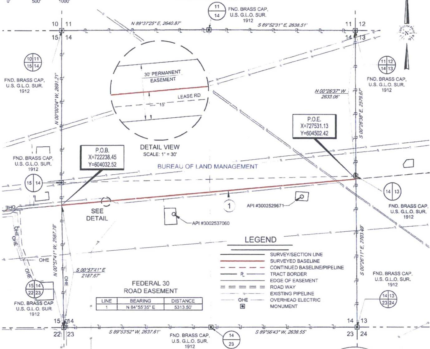
Being a proposed road easement being 30 feet in width, 15 feet left, and 15 feet right of the above platted centerline total line footage containing 5313.50 feet or 322.03 rods, containing 3.66 acres more or less.
