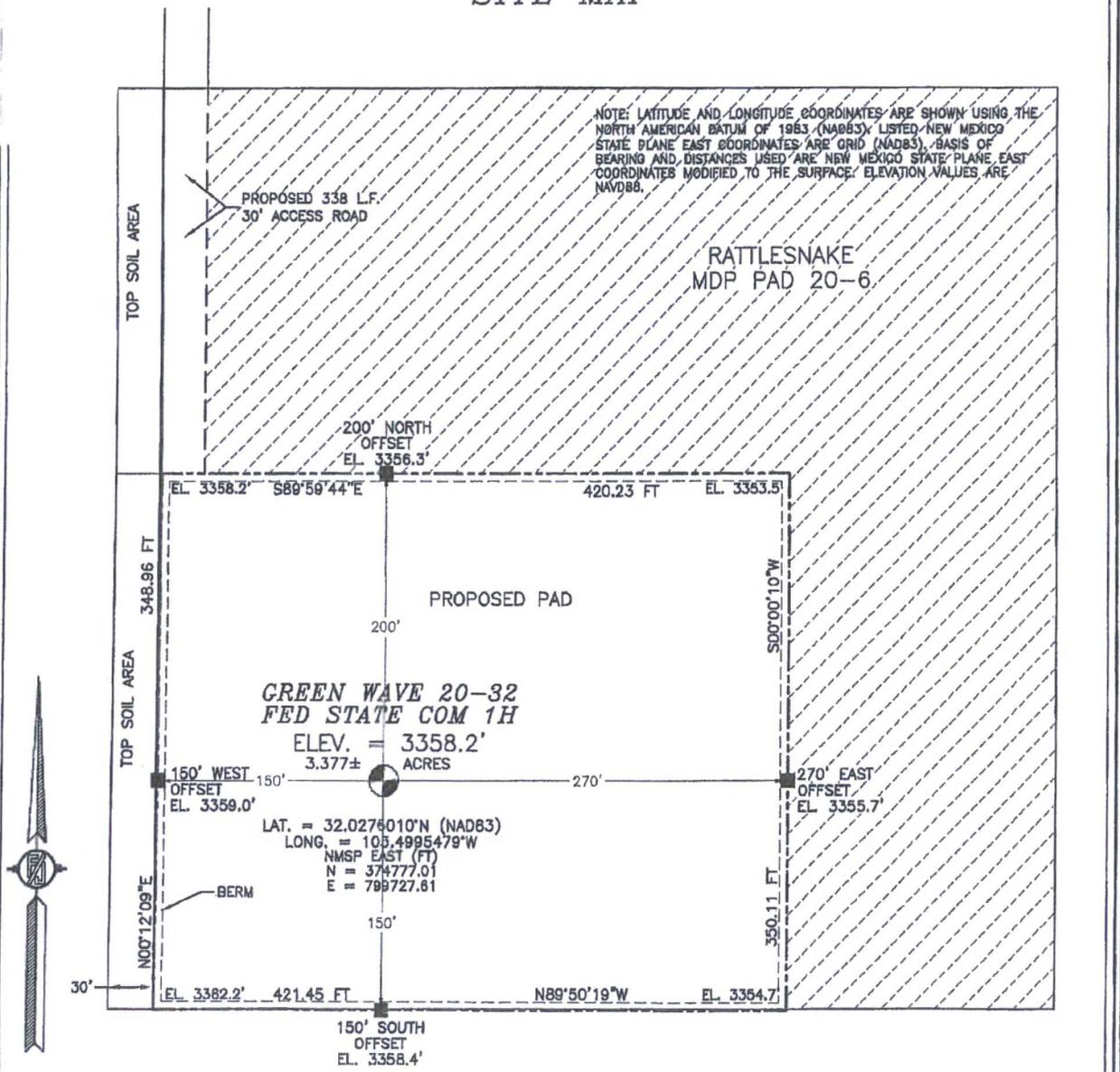
NOTE: LATITUDE AND LONGITUDE COORDINATES ARE SHOWN USING THE NORTH AMERICAN DATUM OF 1983 (NAD83). LISTED NEW MEXICO STATE PLANE EAST COORDINATES ARE GRID (NAD83). BASIS OF BEARING AND DISTANCES USED ARE NEW MEXICO STATE PLANE EAST COORDINATES MODIFIED TO THE SURFACE. ELEVATION VALUES ARE NAVD88.
