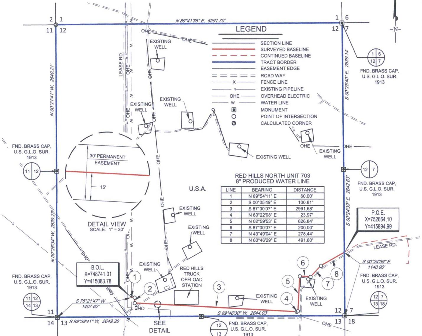
Being a proposed 8-inch water line easement being 30 feet in width, 15 feet left and right of the above platted centerline total line footage containing 4773.54 feet or 289.31 rods, containing 3.29 acres more or less.
