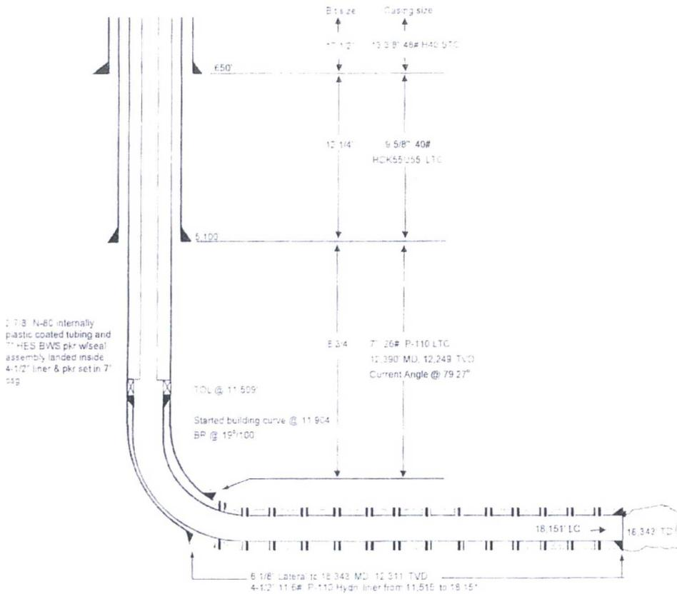
1 7/8" N-80 internally plastic coated tubing and 11 HES BWS pk w/seal assembly landed inside 4-1/2" liner & pk set in 7" casing
