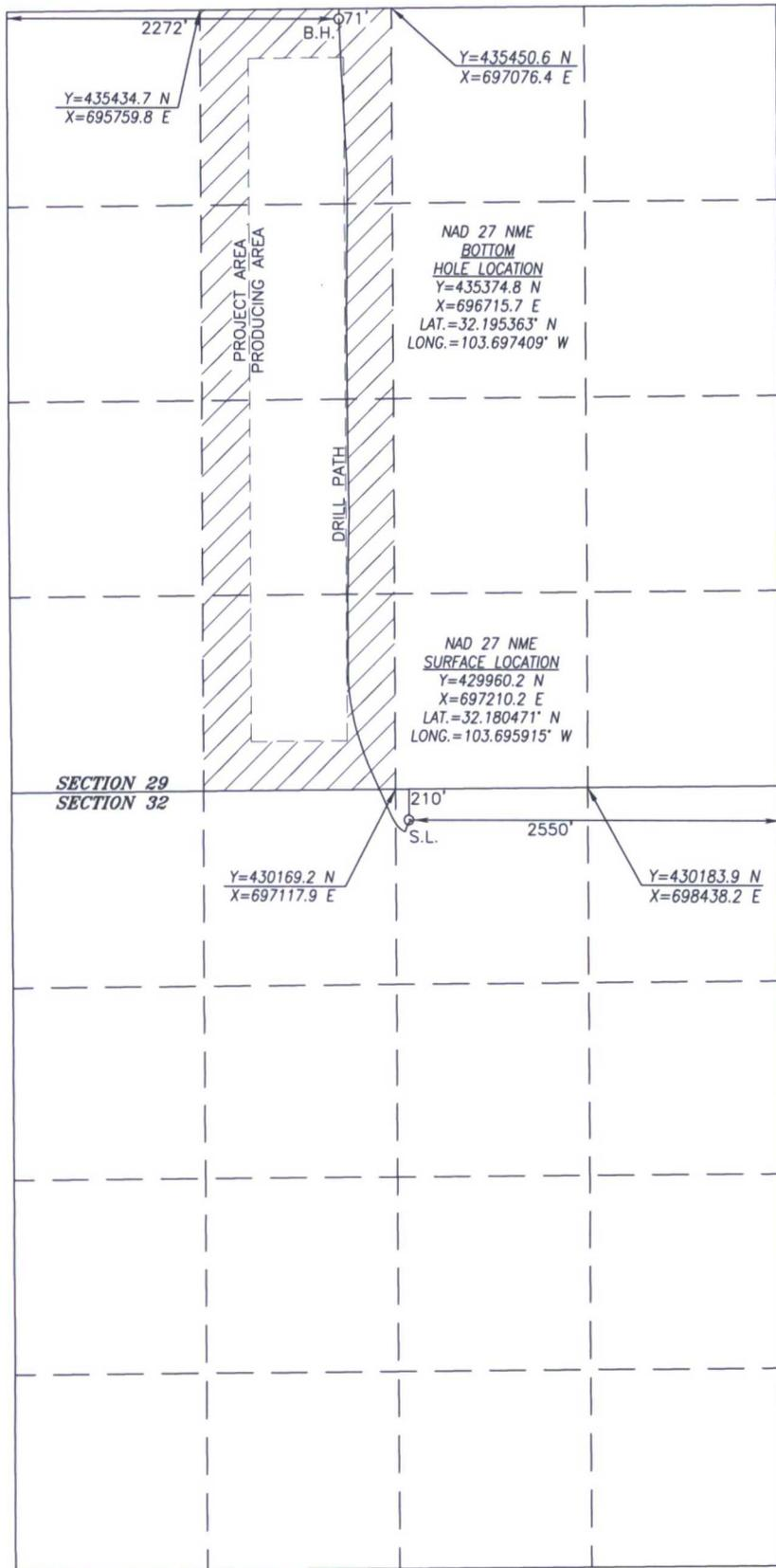
BOREPATH SHOWN HEREON IS BASED ON DIRECTIONAL SURVEY REPORT PROVIDED BY COG OPERATING, LLC FOR THE AZORES FEDERAL #7H SUPPLIED TO HARCROW SURVEYING, LLC ON SEPTEMBER 22, 2016
