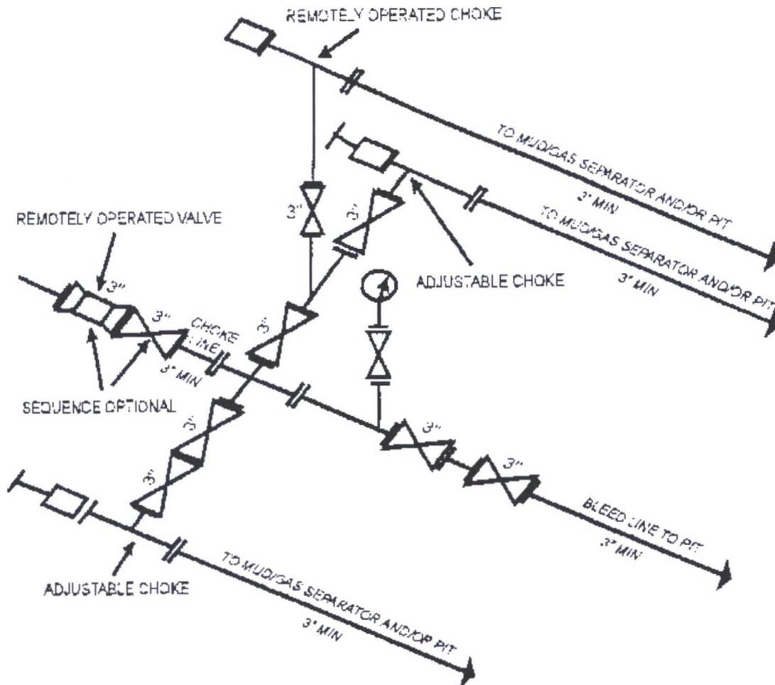
10M AND 15M CHOKE MANIFOLD EQUIPMENT - CONFIGURATION OF CHOKES MAY VARY
