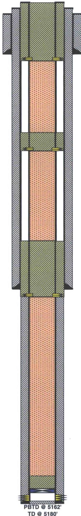
4. PUH & perf @ 341' & sqz 95 sx Class "C" cmt from 341' to surf. Attempt to CIRC 5 1/2" csg to surf. (Surf Shoe & Water Board)
