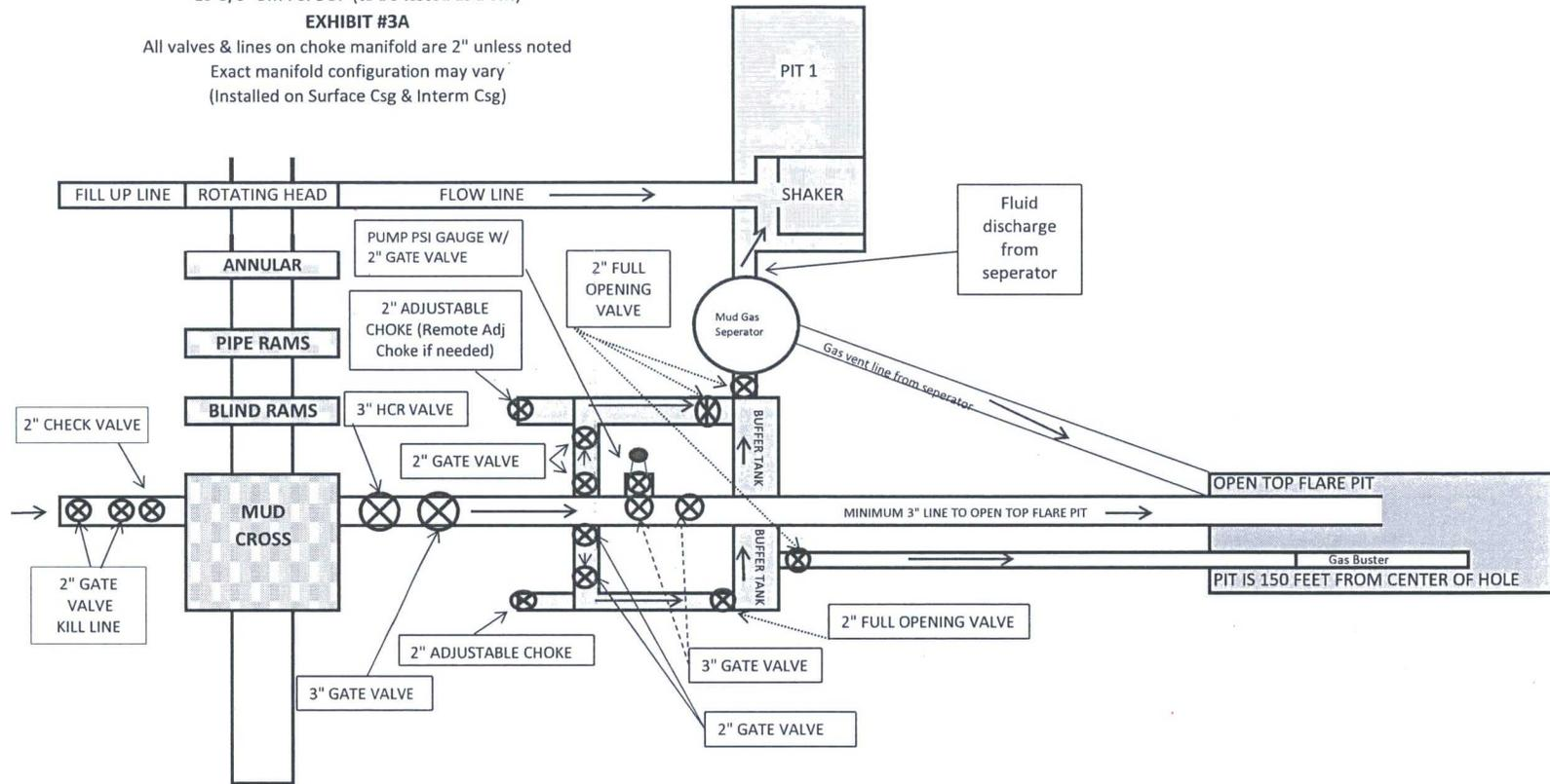
\*\*\* If H2S is encountered in quantities greater than 100ppm, Apache will shut in well & install a remote operated choke \*\*\*
