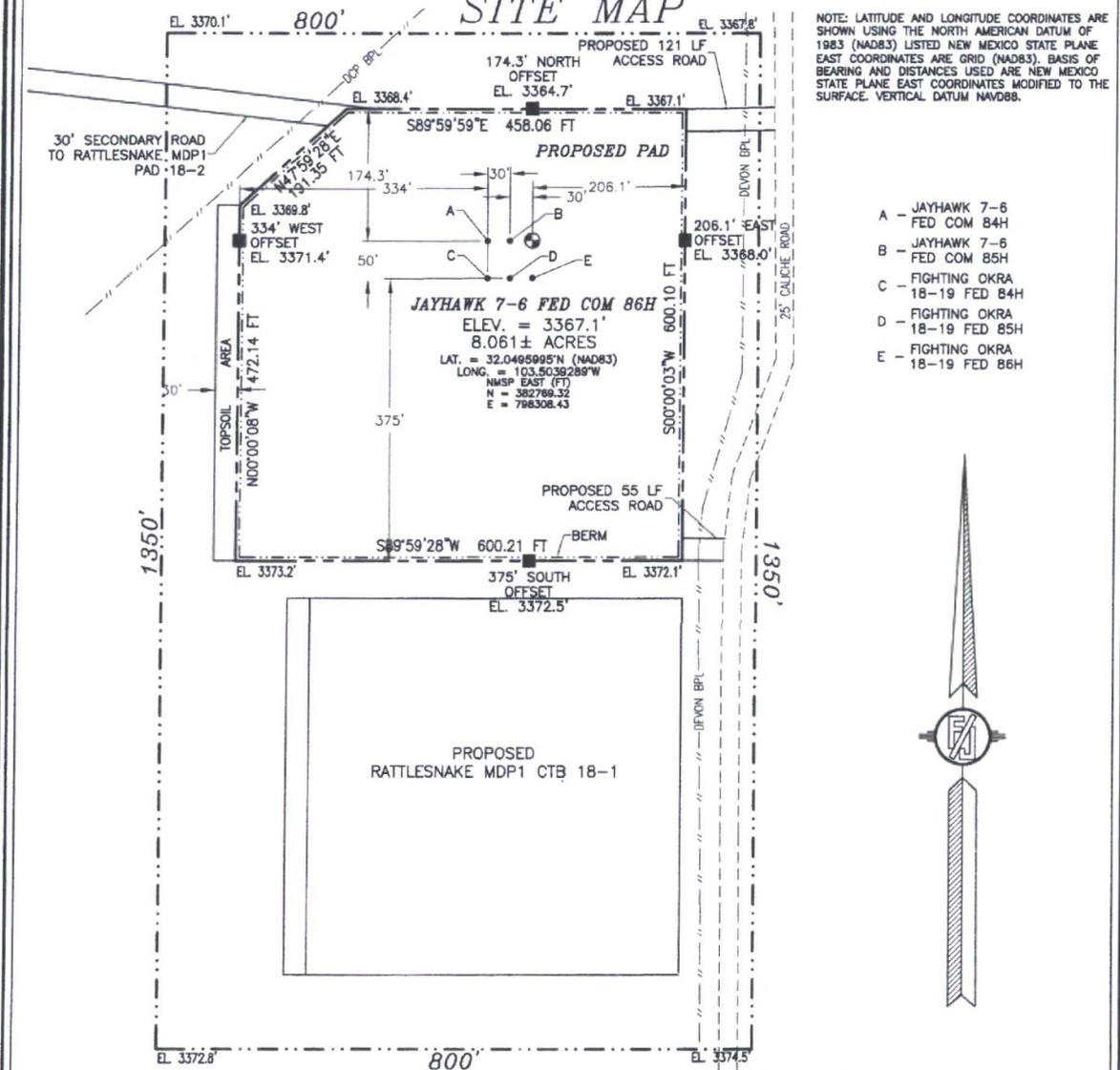
NOTE: LATITUDE AND LONGITUDE COORDINATES ARE SHOWN USING THE NORTH AMERICAN DATUM OF 1983 (NAD83) LISTED NEW MEXICO STATE PLANE EAST COORDINATES ARE GRID (NAD83). BASIS OF BEARING AND DISTANCES USED ARE NEW MEXICO STATE PLANE EAST COORDINATES MODIFIED TO THE SURFACE. VERTICAL DATUM NAVD88.
