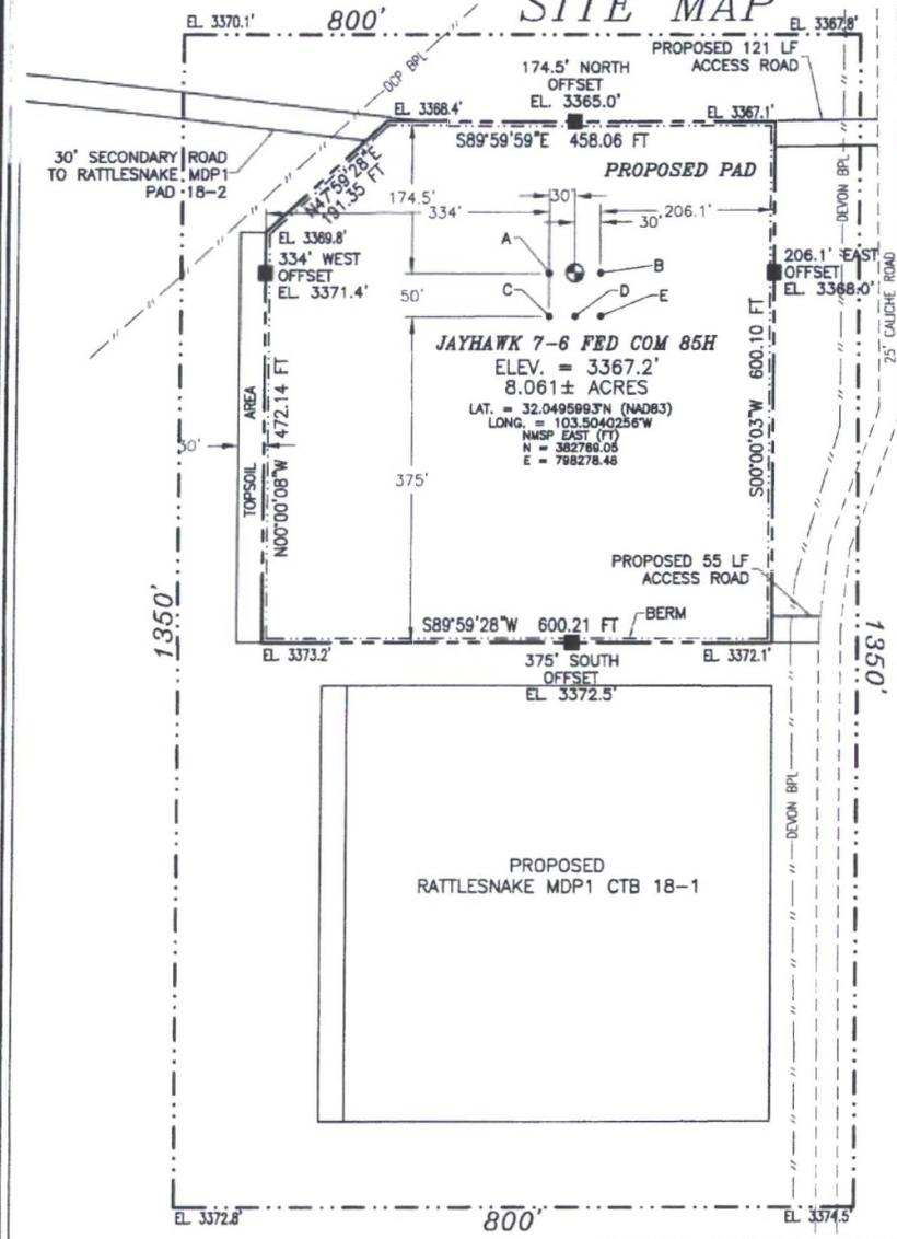
NOTE: LATITUDE AND LONGITUDE COORDINATES ARE SHOWN USING THE NORTH AMERICAN DATUM OF 1983 (NAD83) LISTED NEW MEXICO STATE PLANE EAST COORDINATES ARE GRID (NAD83). BASIS OF BEARING AND DISTANCES USED ARE NEW MEXICO STATE PLANE EAST COORDINATES MODIFIED TO THE SURFACE. VERTICAL DATUM NAVD88.
