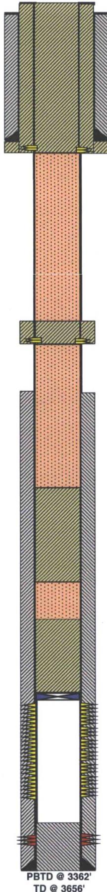
4. PUH & perf @ 450' & sqz 100 sx Class "C" cmt from 450' to surf. Attempt to CIRC 4 1/2" csg to surf. (Surf Shoe & Water Board)
