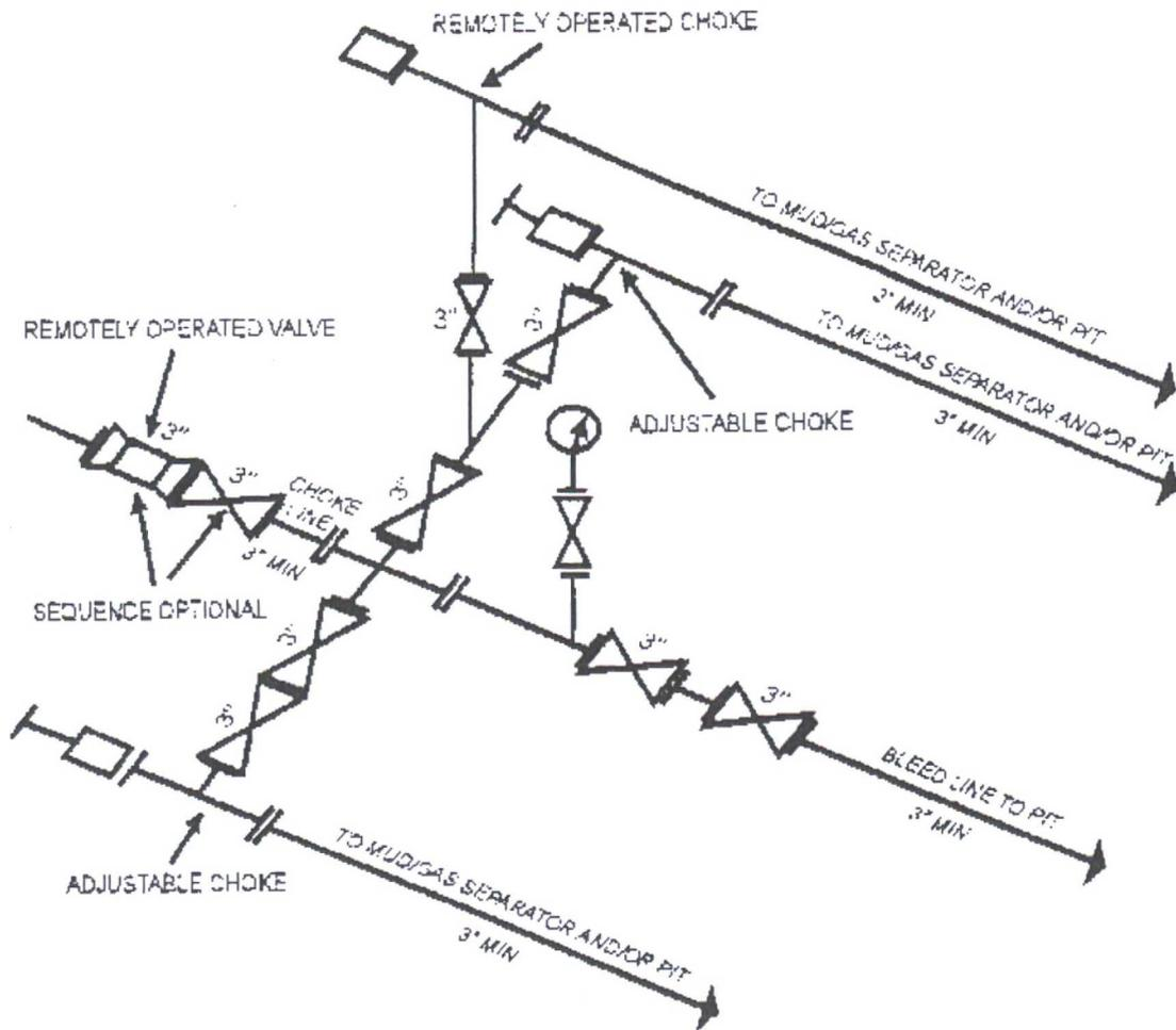
10M AND 15M CHOKE MANIFOLD EQUIPMENT - CONFIGURATION OF CHOKES MAY VARY
