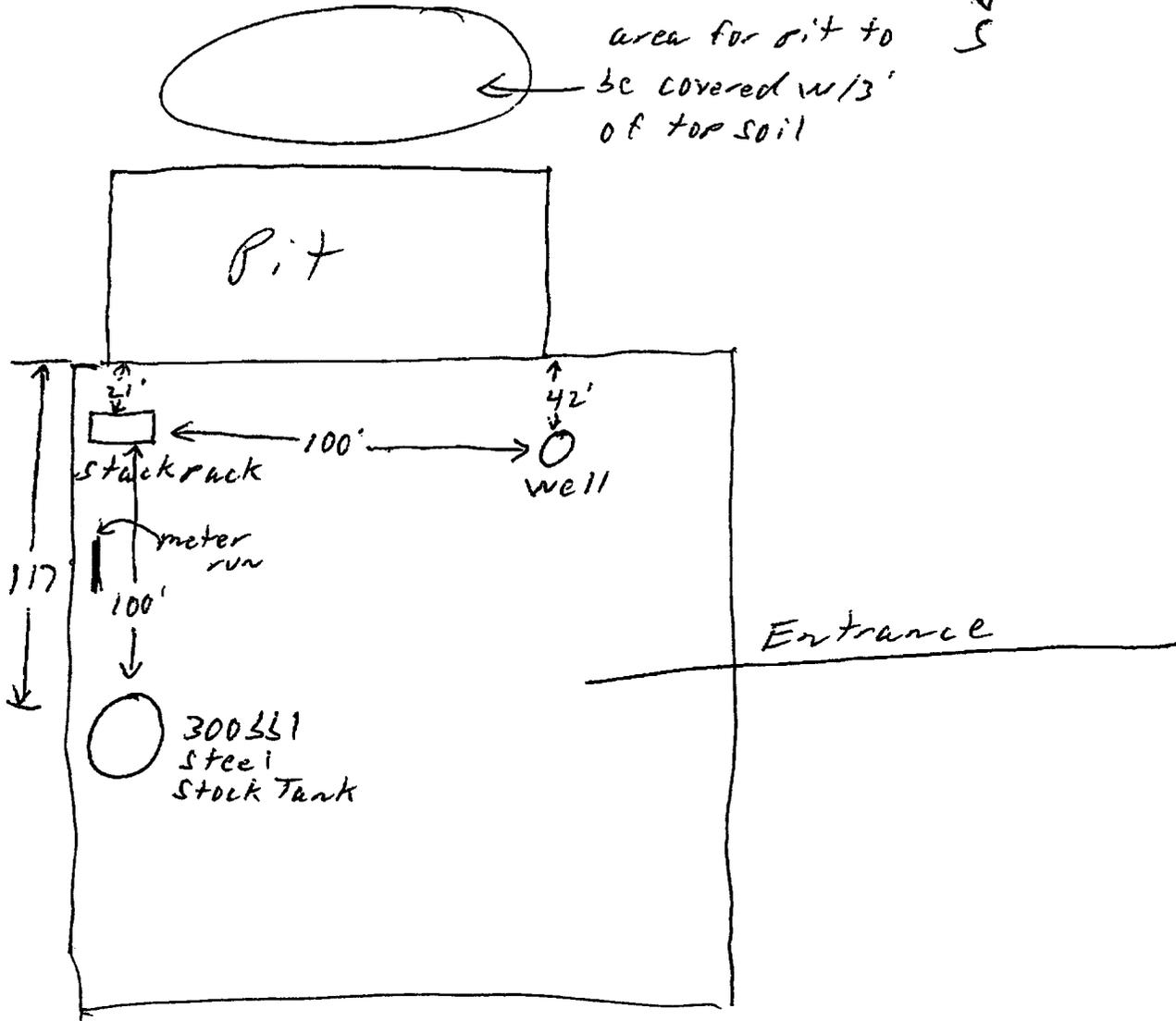
Plan to dig a bury pit 20' wide x 100' long and line w/ plastic. Put cuttings in pit, cover w/ plastic and 3' of fill dirt.
