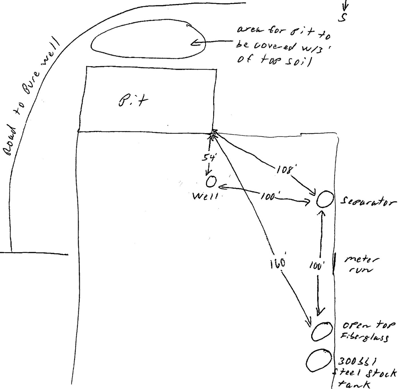
Plan to dig a bury pit 20' wide x 100' long and line w/ plastic. Put cuttings in pit, cover w/ plastic and 3' of fill dirt.
